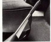
☐ The hand brake is in the right place - between the front seats. Easy to reach for the driver, even with his safety belt on.
