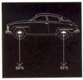
☐ Most of the weight should be at the front, for the sake of stability and road-holding. Both the three cylinder model
