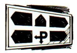
The driver receives advance notice of forthcoming turns from a panel mounted in the centre of the dash. For straight-ahead driving, the centre green arrow is illuminated. Should a right or left turn be needed, a warning buzz will alert the driver. An amber arrow will be illuminated one road before the turn is required, a red arrow will show that the turn is required on the next road available.
